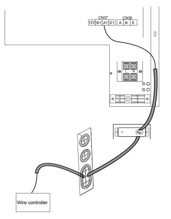
The wire controller line needs to be routed through pipelines or walls.
