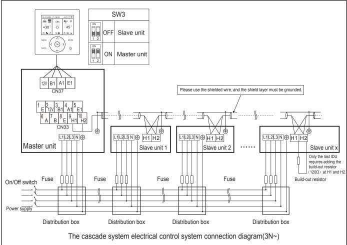
• The cascade function of the system only supports 8 machines at most.
