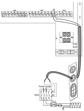
For standard monobloc 16kW, there is no internal backup heater inside the monobloc, but the monobloc can be connected to an external backup heater, as described in the picture below.
