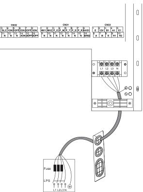
Power Supply Wiring needs to be routed through pipelines or walls.
