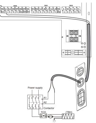
Control signal port of indoor unit: The TBH contains terminals for solar energy , 3-way valve, pump, water tank electric heating , etc. The parts wiring is illustrated below:
