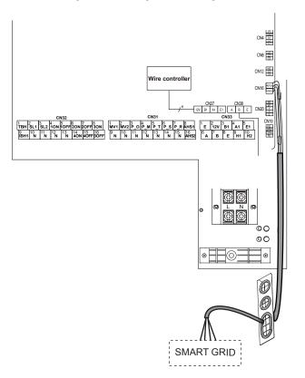
1. When EVU signal is on , and SG signal is on, as long as the DHW mode is set to be valid, heat pump will operate DHW mode priority and the DHW mode setting temperature will be change to  $70^{\circ}$ C. Thwt< $69^{\circ}$ C, the TBH is on,Thwt> $70^{\circ}$ C, the TBH is off.
